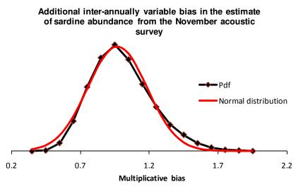
**Figure B.2.** The probability density function for the factors which cause bias in the sardine acoustic survey estimates and which vary inter-annually, calculated by drawing 10 000 samples from the individual probability distribution functions for each source of variable and random error. The normal distribution fitted to this pdf is  $N(0.969, 0.215^2)$ . The CV of this distribution is thus  $\phi_{ac}^{S} = 0.215/0.969 = 0.222$ .
